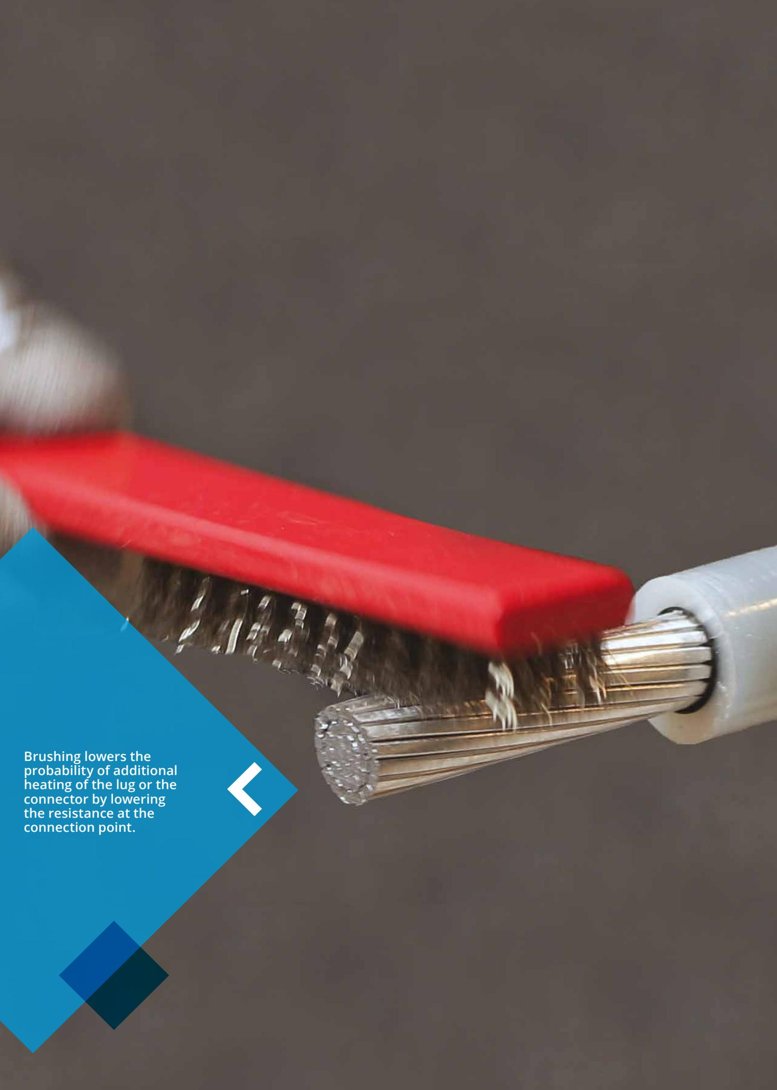
Brushing lowers the probability of additional heating of the lug or the connector by lowering the resistance at the connection point.
