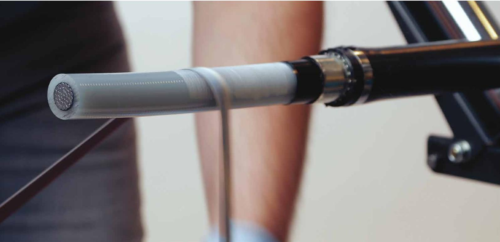
The insulation thickness is defined by the rated voltage of the cable. Cross-linked polyethylene (XLPE) and ethylene propylene rubber (EPR) are common insulation materials.
