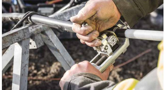
Ensto ST259 is an outer sheath spreading wedge that is also used to help open or remove the outer sheath of single and three-core cables of different constructions.
