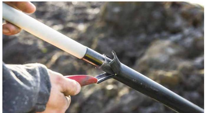
Ensto ST286 is used to spread the outer sheath and/or aluminum laminate. It does not harm the aluminum laminate or semi-conductive layer during spreading.
